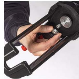
3. Insert and screw down the appropriate plunger discs matching the selected cartridge tray.
