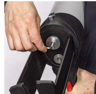
2. Undo the plunger screws and remove the plunger discs.
