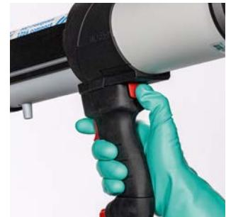
4. Actuate the pressure release button before switching to the next packer and also before any cartridge replacement.
