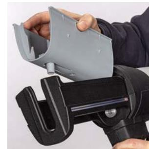
1. Press the cartridge shell upwards and remove it.
