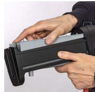
4. Insert the required cartridge tray and press down so that the retaining clips engage.
